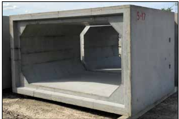
Finished Box Culvert
